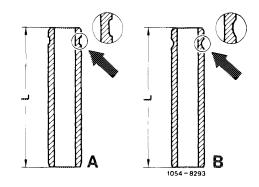
Uprated engines, being of greater valve lift, will only accept the shorter valve guides (B):
