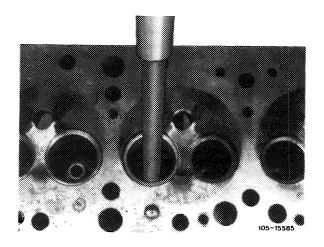
5 If repair stage valve guides are going to be used it is necessary to force appropriate hand broach through basic bore in cylinder head.
