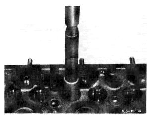
7 Wait until cylinder head has cooled down prior to checking valve guide for firm fit.
